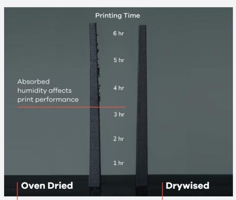
Oven-dried filament (60 hr, 80 °C) quickly absorbs humidity from the environment, negatively affecting print performance.
